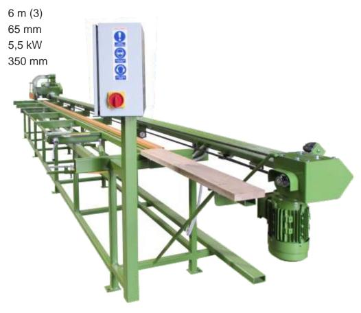
The cutter is equipped with two gears that allow for longitudinal cutting of boards up to 20 and up to 36 cm wide. The use of movable splitting wedges means that the cutter can perform cuts in both directions.
